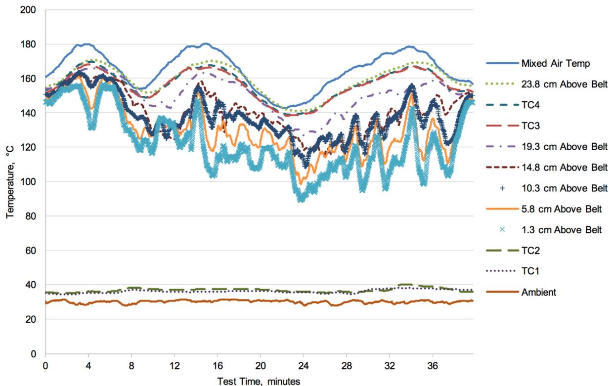
Figure 5. Dryer temperature profile during a dryer characterization test. Beginning at the top, legend entries are arranged from highest to lowest temperature, with the mixed air inlet temperature being highest and the ambient temperature, lowest.
