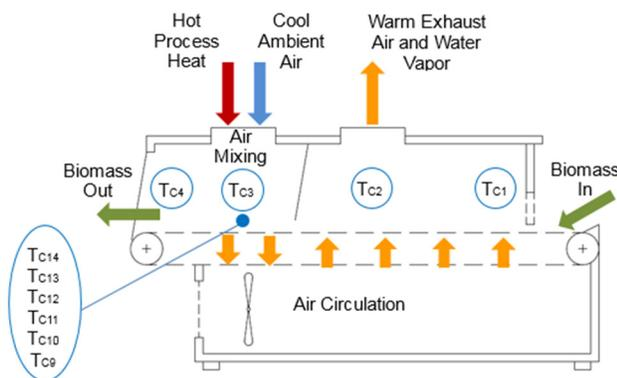
Figure 3. Schematic showing basic belt dryer operation and thermocouple measurement points.
