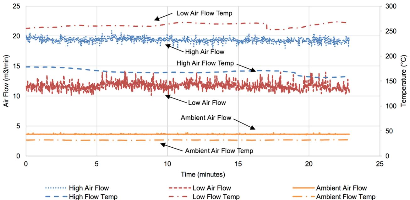
**Figure 4. Air flow and temperature to the dryer.**
