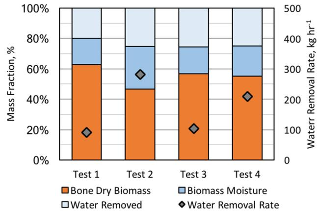
Figure 6. Mass fraction of biomass for each test showing fractions of bone dry biomass, moisture within biomass, and water removed during testing. The water removal rate, shown as diamond markers, is read from the right axis.
