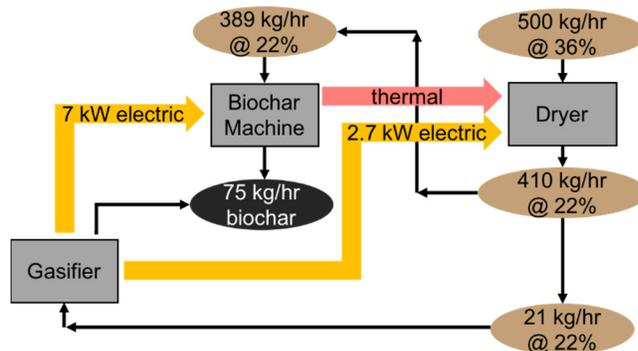
Figure 7. Process flow diagram and measured results for integrated biochar production operation. This diagram includes average values for characteristic operation, but instantaneous conditions will vary depending on specific conditions and flow rates.
